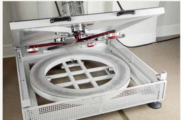
The abrasion is conducted on the Darmstadt machine.
