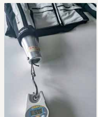
Testing the fastening system
